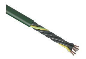
igus continuous flexing control cable, unshielded, 5 conductors (includes ground), 16 AWG (1.50mm2), bare copper, PVC conductor insulation material, black with white numbers and green/yellow ground, PVC jacket, green, cut to length.
