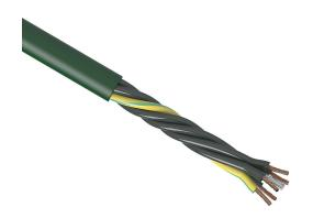
igus continuous flexing control cable, unshielded, 5 conductors (includes ground), 16 AWG (1.50mm2), bare copper, PVC conductor insulation material, black with white numbers and green/yellow ground, PVC jacket, green, cut to length.
