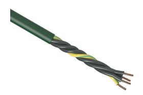
igus continuous flexing control cable, unshielded, 4 conductors (includes ground), 16 AWG (1.50mm2), bare copper, PVC conductor insulation material, black with white numbers and green/yellow ground, PVC jacket, green, cut to length.
