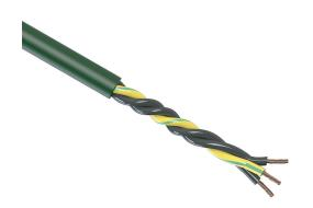
igus continuous flexing control cable, unshielded, 3 conductors (includes ground), 16 AWG (1.50mm2), bare copper, PVC conductor insulation material, black with white numbers and green/yellow ground, PVC jacket, green, cut to length.
