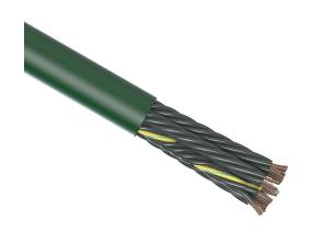
igus continuous flexing control cable, unshielded, 25 conductors (includes ground), 18 AWG (0.75mm2), bare copper, PVC conductor insulation material, black with white numbers and green/yellow ground, PVC jacket, green, cut to length.
