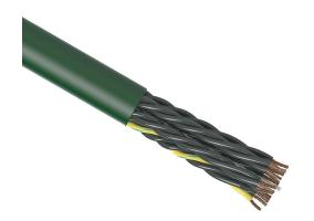
igus continuous flexing control cable, unshielded, 18 conductors (includes ground), 18 AWG (0.75mm2), bare copper, PVC conductor insulation material, black with white numbers and green/yellow ground, PVC jacket, green, cut to length.
