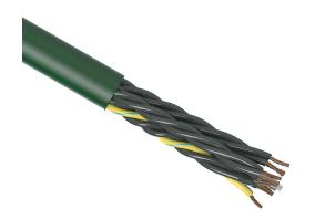
igus continuous flexing control cable, unshielded, 12 conductors (includes ground), 18 AWG (0.75mm2), bare copper, PVC conductor insulation material, black with white numbers and green/yellow ground, PVC jacket, green, cut to length.
