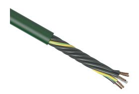
igus continuous flexing control cable, unshielded, 7 conductors (includes ground), 18 AWG (0.75mm2), bare copper, PVC conductor insulation material, black with white numbers and green/yellow ground, PVC jacket, green, cut to length.
