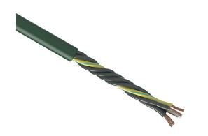
igus continuous flexing control cable, unshielded, 5 conductors (includes ground), 18 AWG (0.75mm2), bare copper, PVC conductor insulation material, black with white numbers and green/yellow ground, PVC jacket, green, cut to length.
