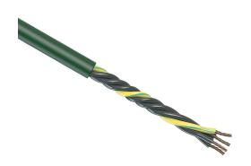
igus continuous flexing control cable, unshielded, 4 conductors (includes ground), 18 AWG (0.75mm2), bare copper, PVC conductor insulation material, black with white numbers and green/yellow ground, PVC jacket, green, cut to length.
