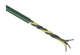
igus continuous flexing control cable, unshielded, 3 conductors (includes ground), 18 AWG (0.75mm2), bare copper, PVC conductor insulation material, black with white numbers and green/yellow ground, PVC jacket, green, cut to length.
