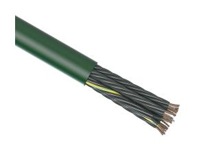
igus continuous flexing control cable, unshielded, 25 conductors (includes ground), 20 AWG (0.50mm2), bare copper, TPE conductor insulation material, black with white numbers and green/yellow ground, PVC jacket, green, cut to length.
