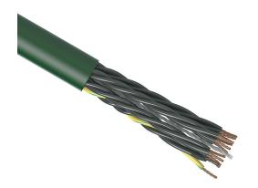
igus continuous flexing control cable, unshielded, 18 conductors (includes ground), 20 AWG (0.50mm2), bare copper, TPE conductor insulation material, black with white numbers and green/yellow ground, PVC jacket, green, cut to length.
