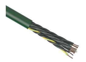
igus continuous flexing control cable, unshielded, 12 conductors (includes ground), 20 AWG (0.50mm2), bare copper, TPE conductor insulation material, black with white numbers and green/yellow ground, PVC jacket, green, cut to length.
