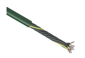
igus continuous flexing control cable, unshielded, 7 conductors (includes ground), 20 AWG (0.50mm2), bare copper, TPE conductor insulation material, black with white numbers and green/yellow ground, PVC jacket, green, cut to length.
