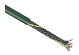
igus continuous flexing control cable, unshielded, 7 conductors (includes ground), 20 AWG (0.50mm2), bare copper, TPE conductor insulation material, black with white numbers and green/yellow ground, PVC jacket, green, cut to length.
