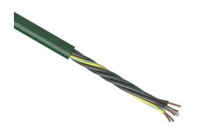
igus continuous flexing control cable, unshielded, 5 conductors (includes ground), 20 AWG (0.50mm2), bare copper, TPE conductor insulation material, black with white numbers and green/yellow ground, PVC jacket, green, cut to length.
