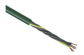
igus continuous flexing control cable, unshielded, 5 conductors (includes ground), 20 AWG (0.50mm2), bare copper, TPE conductor insulation material, black with white numbers and green/yellow ground, PVC jacket, green, cut to length.
