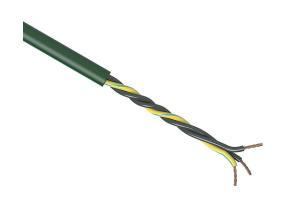
igus continuous flexing control cable, unshielded, 3 conductors (includes ground), 20 AWG (0.50mm2), bare copper, TPE conductor insulation material, black with white numbers and green/yellow ground, PVC jacket, green, cut to length.
