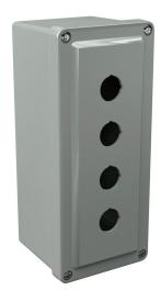
Stahlin CF series pushbutton enclosure, 4 holes, 22mm, NEMA 1/3R/4X/6P/12, 8 x 4 x 4in (HxWxD), wall mount, fiberglass reinforced polyester, gray, screw cover.
