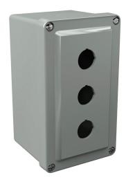
Stahlin CF series pushbutton enclosure, 3 holes, 22mm, NEMA 1/3R/4X/6P/12, 6 x 4 x 4in (HxWxD), wall mount, fiberglass reinforced polyester, gray, screw cover.
