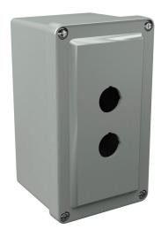
Stahlin CF series pushbutton enclosure, 2 holes, 22mm, NEMA 1/3R/4X/6P/12, 6 x 4 x 4in (HxWxD), wall mount, fiberglass reinforced polyester, gray, screw cover.
