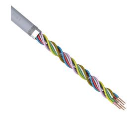
igus continuous flexing control and signal cable, shielded, 4 twisted pairs, 20 AWG (0.50mm2), 28-stranded, bare copper, TPE conductor insulation material, PUR jacket, gray, cut to length.
