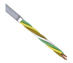
igus continuous flexing control and signal cable, shielded, AWM, 2 twisted pairs, 20 AWG (0.50mm2), bare copper, TPE conductor insulation material, pair 1: white and brown and pair 2: green and yellow, PUR jacket, gray, cut to length.
