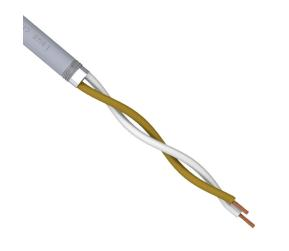
igus continuous flexing control and signal cable, shielded, AWM, 1 twisted pair, 20 AWG (0.50mm2), bare copper, TPE conductor insulation material, white and brown, PUR jacket, gray, cut to length.
