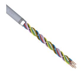
igus continuous flexing control and signal cable, shielded, 4 twisted pairs, 24 AWG (0.25mm2), 32-stranded, bare copper, TPE conductor insulation material, PUR jacket, gray, cut to length.
