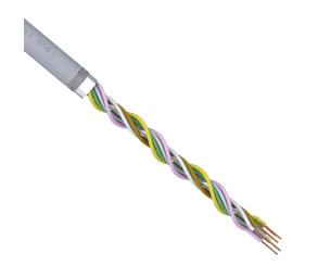
igus continuous flexing control and signal cable, shielded, AWM, 3 twisted pairs, 24 AWG (0.25mm2), bare copper, TPE conductor insulation material, pair 1: white and brown, pair 2: green and yellow and pair 3: grey and pink, PUR jacket, gray, cut to length.
