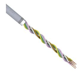
igus continuous flexing control and signal cable, shielded, AWM, 3 twisted pairs, 24 AWG (0.25mm2), bare copper, TPE conductor insulation material, pair 1: white and brown, pair 2: green and yellow and pair 3: grey and pink, PUR jacket, gray, cut to length.
