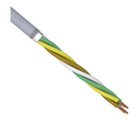
igus continuous flexing control and signal cable, shielded, AWM, 2 twisted pairs, 24 AWG (0.25mm2), bare copper, TPE conductor insulation material, pair 1: white and brown and pair 2: green and yellow, PUR jacket, gray, cut to length.
