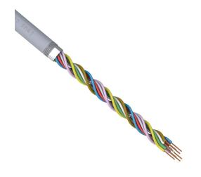
igus continuous flexing control and signal cable, shielded, 4 twisted pairs, 20 AWG (0.50mm2), 28-stranded, bare copper, TPE conductor insulation material, PVC jacket, gray, cut to length.
