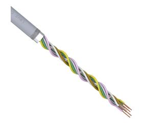
igus continuous flexing control and signal cable, shielded, AWM, 3 twisted pairs, 20 AWG (0.50mm2), bare copper, TPE conductor insulation material, pair 1: white and brown, pair 2: green and yellow and pair 3: grey and pink, PVC jacket, gray, cut to length.
