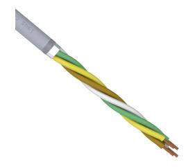
igus continuous flexing control and signal cable, shielded, AWM, 2 twisted pairs, 20 AWG (0.50mm2), bare copper, TPE conductor insulation material, pair 1: white and brown and pair 2: green and yellow, PVC jacket, gray, cut to length.
