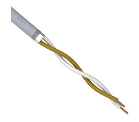
igus continuous flexing control and signal cable, shielded, AWM, 1 twisted pair, 20 AWG (0.50mm2), bare copper, TPE conductor insulation material, white and brown, PVC jacket, gray, cut to length.
