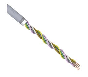
igus continuous flexing control and signal cable, shielded, AWM, 3 twisted pairs, 22 AWG (0.34mm2), bare copper, TPE conductor insulation material, pair 1: white and brown, pair 2: green and yellow and pair 3: grey and pink, PVC jacket, gray, cut to length.
