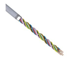
igus continuous flexing control and signal cable, shielded, 4 twisted pairs, 24 AWG (0.25mm2), 32-stranded, bare copper, TPE conductor insulation material, PVC jacket, gray, cut to length.
