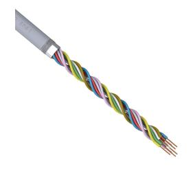
igus continuous flexing control and signal cable, shielded, 4 twisted pairs, 24 AWG (0.25mm2), 32-stranded, bare copper, TPE conductor insulation material, PVC jacket, gray, cut to length.
