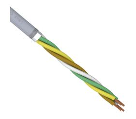
igus continuous flexing control and signal cable, shielded, AWM, 2 twisted pairs, 24 AWG (0.25mm2), bare copper, TPE conductor insulation material, pair 1: white and brown and pair 2: green and yellow, PVC jacket, gray, cut to length.
