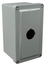
Stahlin CF series pushbutton enclosure, 1 hole, 30mm, NEMA 1/3R/4X/6P/12, 6 x 4 x 4in (HxWxD), wall mount, fiberglass reinforced polyester, gray, screw cover.
