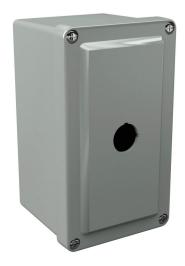
Stahlin CF series pushbutton enclosure, 1 hole, 22mm, NEMA 1/3R/4X/6P/12, 6 x 4 x 4in (HxWxD), wall mount, fiberglass reinforced polyester, gray, screw cover.
