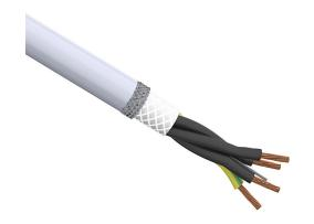
igus continuous flexing control cable, shielded, 4 conductors (includes ground), 12 AWG (4mm2), bare copper, PVC/Nylon conductor insulation material, black with white numbers and green/yellow ground, PVC jacket, gray, cut to length.
