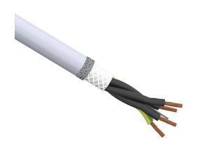
igus continuous flexing control cable, shielded, 4 conductors (includes ground), 14 AWG (2.50mm2), bare copper, PVC/Nylon conductor insulation material, black with white numbers and green/yellow ground, PVC jacket, gray, cut to length.
