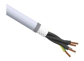
igus continuous flexing control cable, shielded, 4 conductors (includes ground), 16 AWG (1.50mm2), bare copper, PVC/Nylon conductor insulation material, black with white numbers and green/yellow ground, PVC jacket, gray, cut to length.
