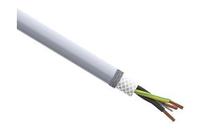
igus continuous flexing control cable, shielded, 3 conductors (includes ground), 16 AWG (1.50mm2), bare copper, PVC/Nylon conductor insulation material, black with white numbers and green/yellow ground, PVC jacket, gray, cut to length.
