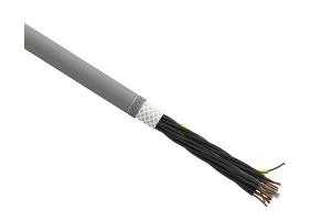
igus continuous flexing control cable, shielded, 18 conductors (includes ground), 18 AWG (0.75mm2), bare copper, PVC/Nylon conductor insulation material, black with white numbers and green/yellow ground, PVC jacket, gray, cut to length.
