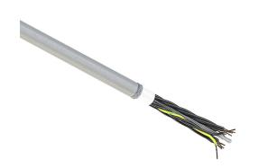
igus continuous flexing control cable, shielded, 12 conductors (includes ground), 18 AWG (0.75mm2), bare copper, PVC/Nylon conductor insulation material, black with white numbers and green/yellow ground, PVC jacket, gray, cut to length.
