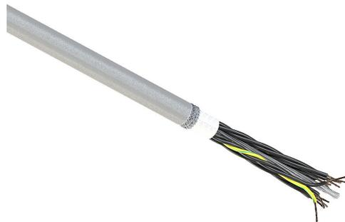
igus continuous flexing control cable, shielded, 12 conductors (includes ground), 18 AWG (0.75mm<sup>2</sup>), bare copper, PVC/Nylon conductor insulation material, black with white numbers and green/yellow ground, PVC jacket, gray, cut to length.
