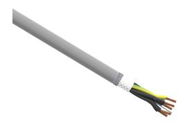
igus continuous flexing control cable, shielded, 5 conductors (includes ground), 18 AWG (0.75mm2), bare copper, PVC/Nylon conductor insulation material, black with white numbers and green/yellow ground, PVC jacket, gray, cut to length.
