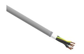
igus continuous flexing control cable, shielded, 5 conductors (includes ground), 18 AWG (0.75mm2), bare copper, PVC/Nylon conductor insulation material, black with white numbers and green/yellow ground, PVC jacket, gray, cut to length.
