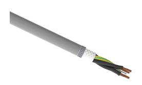
igus continuous flexing control cable, shielded, 4 conductors (includes ground), 18 AWG (0.75mm2), bare copper, PVC/Nylon conductor insulation material, black with white numbers and green/yellow ground, PVC jacket, gray, cut to length.
