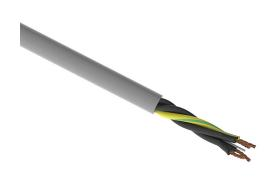
igus continuous flexing control cable, unshielded, 4 conductors (includes ground), 12 AWG (4mm2), bare copper, PVC/Nylon conductor insulation material, black with white numbers and green/yellow ground, PVC jacket, gray, cut to length.
