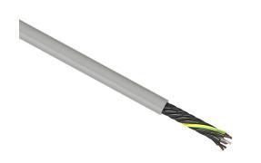
igus continuous flexing control cable, unshielded, 7 conductors (includes ground), 14 AWG (2.50mm2), bare copper, PVC/Nylon conductor insulation material, black with white numbers and green/yellow ground, PVC jacket, gray, cut to length.
