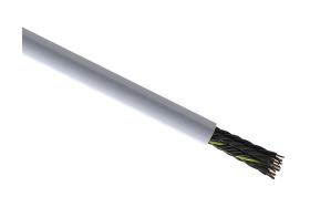
igus continuous flexing control cable, unshielded, 18 conductors (includes ground), 16 AWG (1.50mm2), bare copper, PVC/Nylon conductor insulation material, black with white numbers and green/yellow ground, PVC jacket, gray, cut to length.
