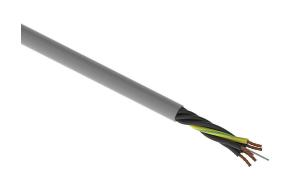
igus continuous flexing control cable, unshielded, 5 conductors (includes ground), 16 AWG (1.50mm2), bare copper, PVC/Nylon conductor insulation material, black with white numbers and green/yellow ground, PVC jacket, gray, cut to length.
