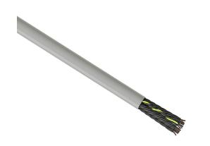
igus continuous flexing control cable, unshielded, 25 conductors (includes ground), 18 AWG (0.75mm2), bare copper, PVC/Nylon conductor insulation material, black with white numbers and green/yellow ground, PVC jacket, gray, cut to length.
