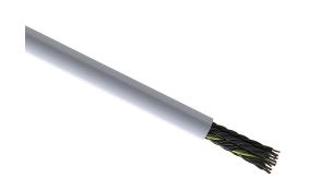
igus continuous flexing control cable, unshielded, 18 conductors (includes ground), 18 AWG (0.75mm2), bare copper, PVC/Nylon conductor insulation material, black with white numbers and green/yellow ground, PVC jacket, gray, cut to length.
