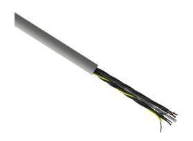
igus continuous flexing control cable, unshielded, 12 conductors (includes ground), 18 AWG (0.75mm2), bare copper, PVC/Nylon conductor insulation material, black with white numbers and green/yellow ground, PVC jacket, gray, cut to length.
