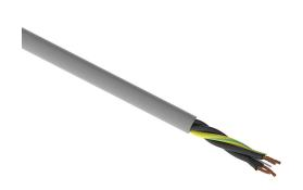
igus continuous flexing control cable, unshielded, 4 conductors (includes ground), 18 AWG (0.75mm2), bare copper, PVC/Nylon conductor insulation material, black with white numbers and green/yellow ground, PVC jacket, gray, cut to length.
